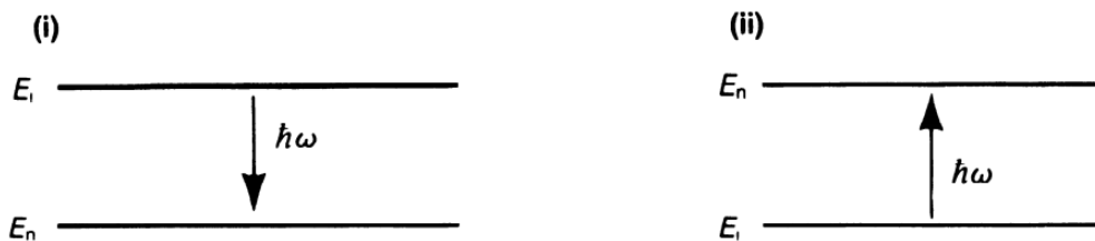
(i) Stimulated emission: Quantum-mechanical system gives up \hbar\omega to V (possible only if initial state is excited). (ii) Absorption: Quantum mechanical system receives \hbar\omega from V and ends up as an excited state.
