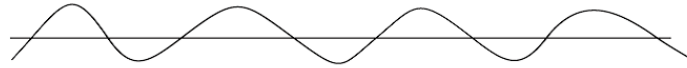
A particle with well-defined momentum p is described by a sinusoidal wave extending from x = -\infty to +\infty . Here \Delta p \rightarrow 0 but \Delta x \rightarrow \infty
